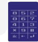
Rotating Keypad (To Prevent Surface Analysis)
