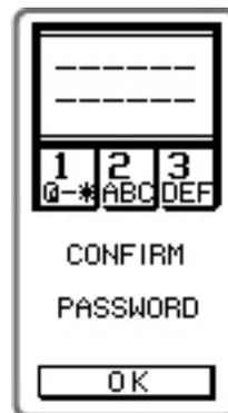
**Step 10:** Press the touch screen 8 times randomly to initiate the seed key generation process. The seed key is used to make each drive unique.
